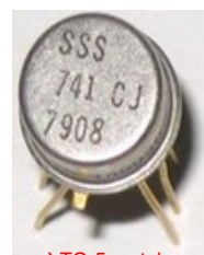
(c) TO-5 metal can 8-Leads package
